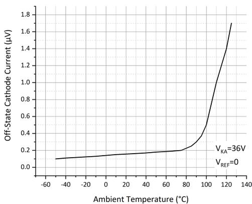
Figure 8: Off-State Cathode Current vs. Ambient Temperature
