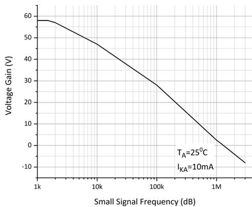
**Figure 10: Small-Signal Voltage Amplification vs Frequency**
