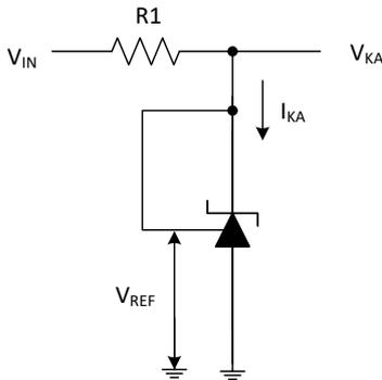
Figure 1: Test Circuit for  $V_{\text{KA}}=V_{\text{ref}}$
