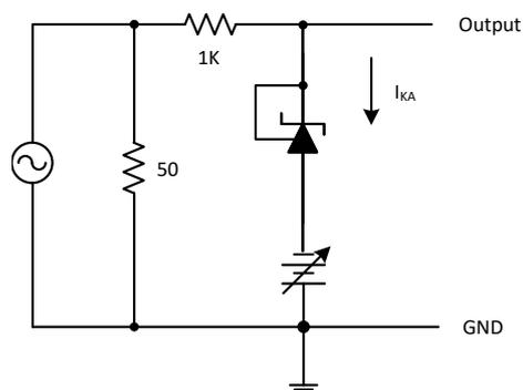
**Figure 13: Test Circuit for Reference Impedance**
