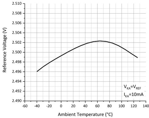
Figure 4: Reference Voltage vs Free-Air Temperature
