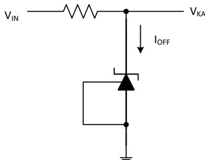
Figure 3: Test Circuit for  $I_{\text{off}}$
