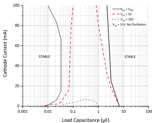
**Figure 14: Stability Boundary Conditions vs. Load Capacitance**
