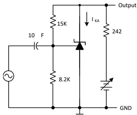
**Figure 11: Test Circuit for Voltage Amplification**
