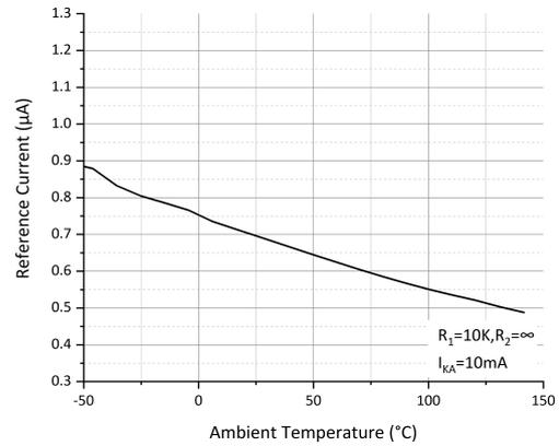
Figure 5: Reference Current vs Free-Air Temperature
