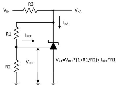
Figure 2: Test Circuit for  $V_{\text{KA}}>V_{\text{ref}}$
