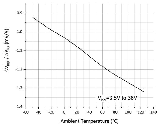
Figure 9: Ratio of Delta Reference Voltage to the Ratio of Delta Cathode Voltage
