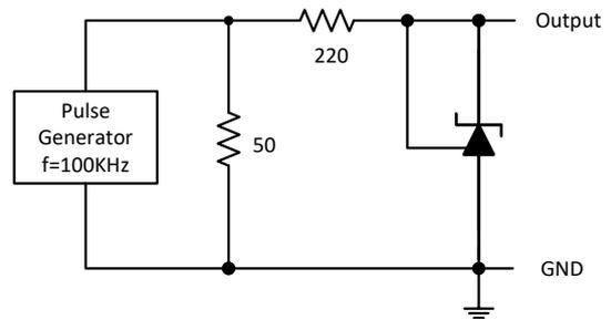
**Figure 17: Test Circuit for Pulse Response**
