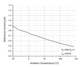
Figure 5: Reference Current vs Free-Air Temperature
