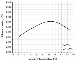
Figure 4: Reference Voltage vs Free-Air Temperature Fig
