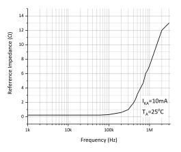
Figure 12: Reference Impedance vs Frequency
