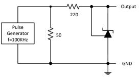
Figure 17: Test Circuit for Pulse Response
