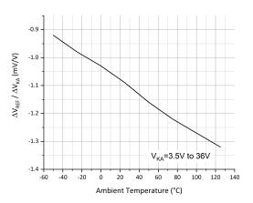
Figure 9: Ratio of Delta Reference Voltage to the Ratio of Delta Cathode Voltage
