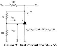
Figure 2: Test Circuit for V<sub>KA</sub>>V<sub>ref</sub>
