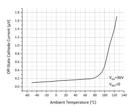
Figure 8: Off-State Cathode Current vs. Ambient Temperature
