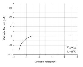
Figure 6: Cathode Current vs Cathode Voltage
