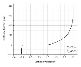
Figure 7: Cathode Current vs. Cathode Voltage
