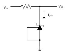
Figure 3: Test Circuit for I<sub>off</sub>
