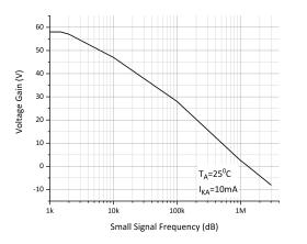
Figure 10: Small-Signal Voltage Amplification vs Frequency
