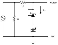
Figure 13: Test Circuit for Reference Impedance
