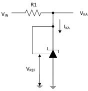
Figure 1: Test Circuit for V<sub>KA</sub>=V<sub>ref</sub>
