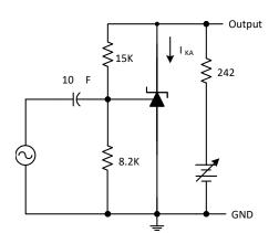
Figure 11: Test Circuit for Voltage Amplification
